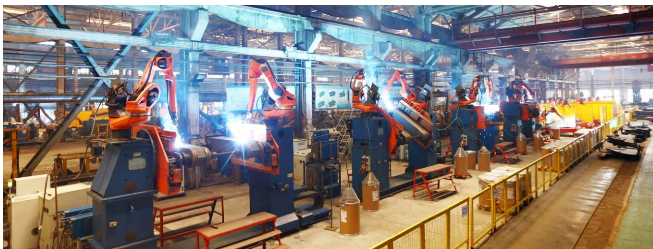
The connecting-rod robot production line of the structural branch of China Coal Beijing Coal Mining Machinery Co., Ltd., widely used in the welding of various hydraulic support connecting rods
